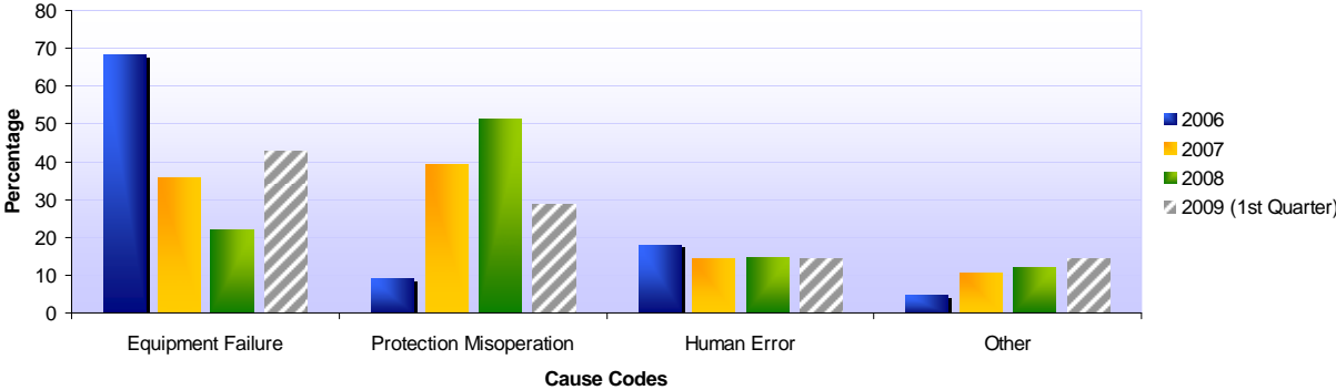
Bulk Power Disturbances by Cause and Year (2006-2009)
